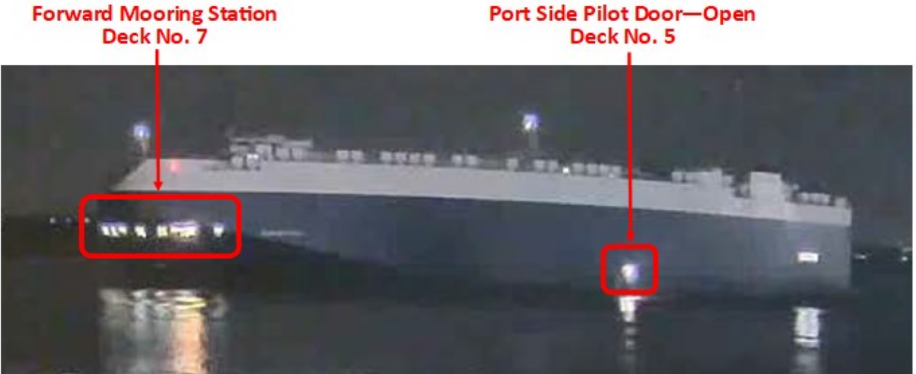
Figure 9. Pilot door condition on outbound transit from Jacksonville September 6, 2019 from JAXPORT CCTV footage
